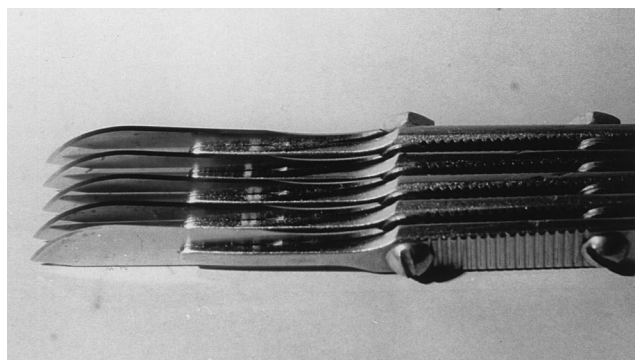
FIG. 1. Five Bard-Parker surgical knives bolted together for making cuts.
