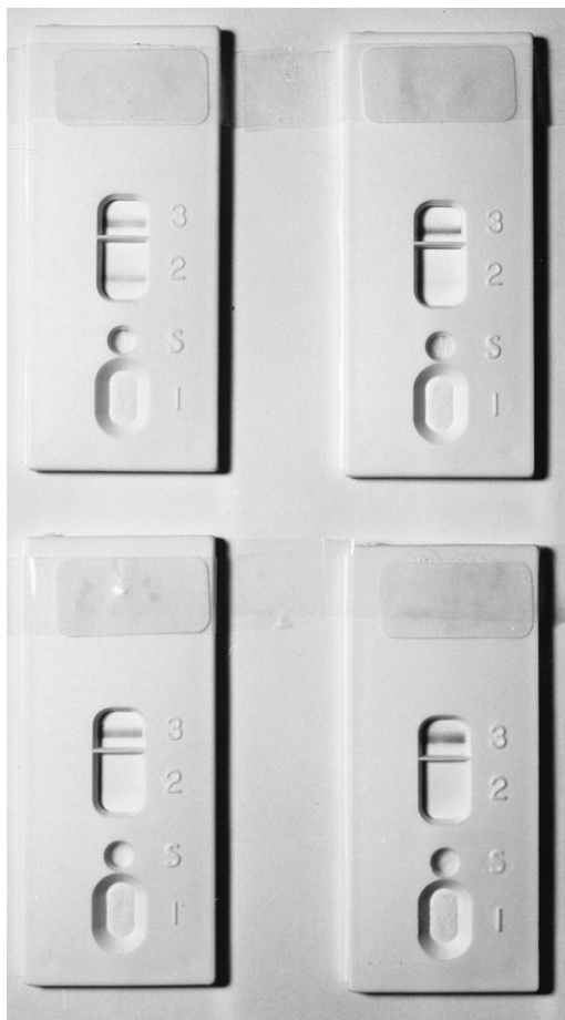
FIG. 1. Photo series of representative negative (lower right), faint (lower left), thin (upper right), and thick (upper left) band results of CLOser. 1, developer well; S, sample well; 2, test window; 3, control window. The grades of the colored band in the test window were defined as follows: thick band, line apparent and usually wider than 1 mm; thin band, line less apparent but confidently visible and usually \leq 1 mm wide; and faint band, only a shade of purple seen without a distinct colored band.
