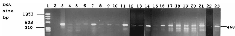
FIG. 5. Agarose gel electrophoresis of PCR-amplified products of the E. risticii 16S rRNA gene from the blood and feces of naturally infected horses. Lane 1, Hae III-digested \phi X174RF DNA; lane 2, negative control (no template); lane 3, positive control (DNA from purified E. risticii ); lanes 4 to 20, DNA purified from the blood of horses Bi, Al, Jo, Sa, Ro, Bl, Mg, So, Ta, Pa, Cy, Su, Hi, Cl, Io, Se, and Li, respectively; lanes 21 to 23, DNA purified from feces of horses Al, Sa, and Ar, respectively.
