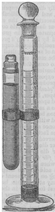
The micro-saccharimeter, as described in the text. The shading of the side-tube indicates the ferric acetate standard. The darker shading at the bottom of the graduated tube shows the saccharine fluid, darkened by boiling with picric acid and potash, and occupying ten divisions before dilution.
