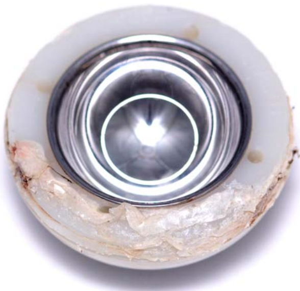
Fig. 1 Retrieved Metasul ® liner with a protruded edge of the inlay has damage to the polyethylene caused by impingement.
