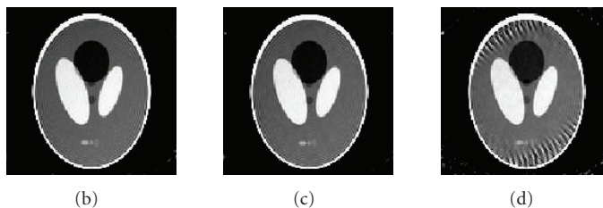
FIGURE 9: Effect of number of interleaves and sampling densities. In (a), PDM is plotted as a function of the sampling densities from 40% to 100% and 6 different numbers of interleaves. Other conditions (Voronoi method, conventional regridding, noise-free) were held constant. Images in (b), (c), and (d) correspond to 100% sample, 70% sample, and 40% sample and 21 interleaves, respectively, as indicated.
