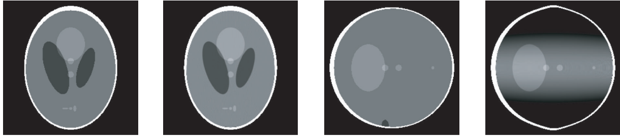
FIGURE 1: 3D Shepp-Logan phantom with total CB angle 36^\circ . From left to right: horizontal mid-plane of the reference phantom, horizontal mid-plane of the reconstruction with the FDK algorithm, vertical plane of the reference phantom, and vertical plane of the FDK reconstruction.
