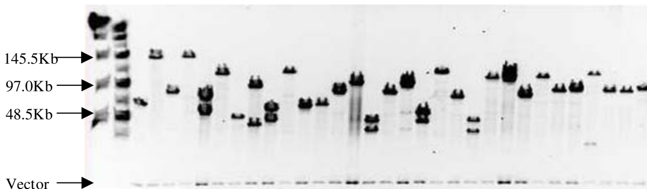
Figure 1 DNA analysis of 31 random BAC clones from the L. calcarifer Hind III BAC library by pulse-field gel electrophoresis. DNA samples digested with Not I were separated on 1% agarose gel in 0.5 × TBE buffer for 16 h under the following conditions: ramp pulse time of 5–15 s at 6 V/cm, temperature at 14°C. Markers used are Lambda Ladder PFG Marker (outside lanes) and MidRange II PFG Marker (NEB, SG, Singapore). The 8 kb common band is the pCC1BAC Vector (Epicentre, WI, USA).
