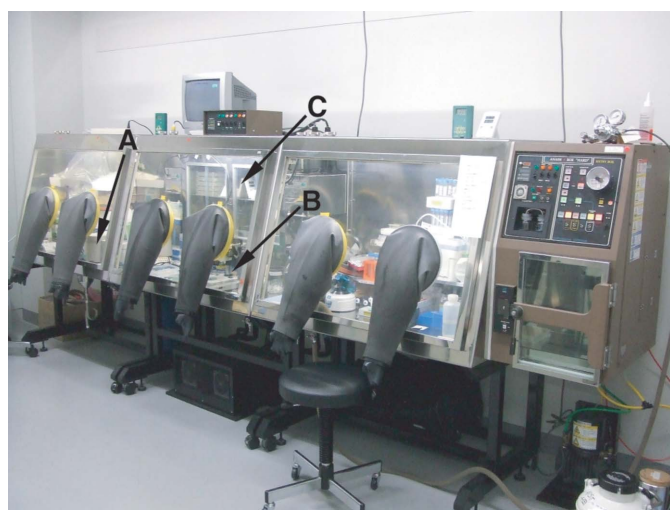
Figure 1 The anaerobic chamber used in the present study. It includes a UV–Vis spectrometer (A), a microscope with CCD (B) and an incubator for crystallization (C) in the anaerobic chamber.
