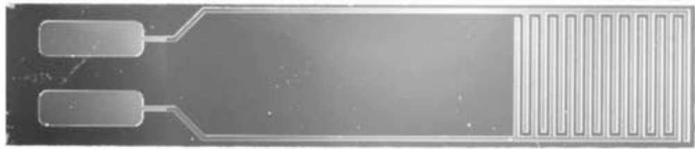
Fig. 10. IDE structure for Impedance spectroscopy test. The width of spacing as well as the interdigitated electrodes was 130\ \mu\text{m} .
