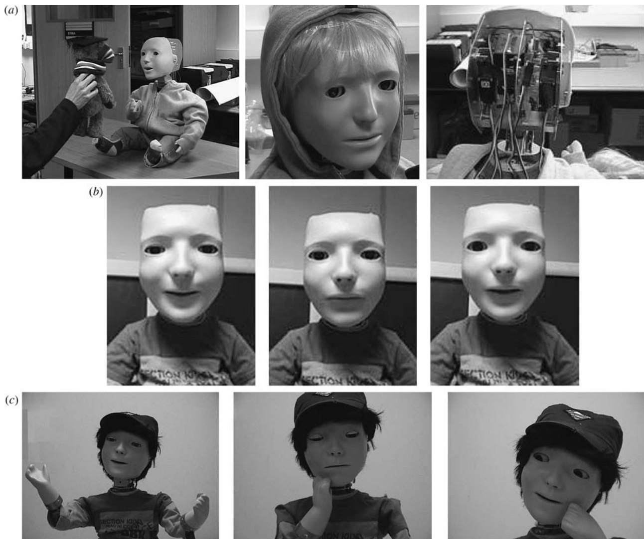
Figure 3. Experimental humanoid robot platform for the study of synchronization, turn-taking and interaction games inspired by child development. Kaspar, a child-sized humanoid robot developed by the Adaptive Systems Research Group at the University of Hertfordshire. (a) Kaspar has a minimally expressive head with eight degrees of freedom in the neck, eyes, eyelids and mouth. The face is a silicon rubber mask, which is supported on an aluminium frame. It has two degrees of freedom in the eyes fitted with video cameras and a mouth capable of opening and smiling. It has six degrees of freedom in the arms and hand and is thus able to show a variety of different expressions. (b) Kaspar's expressions: happy; neutral; and surprised (Blow et al. 2006). (c) Some of Kaspar's expressions using movements in the head and arms.
