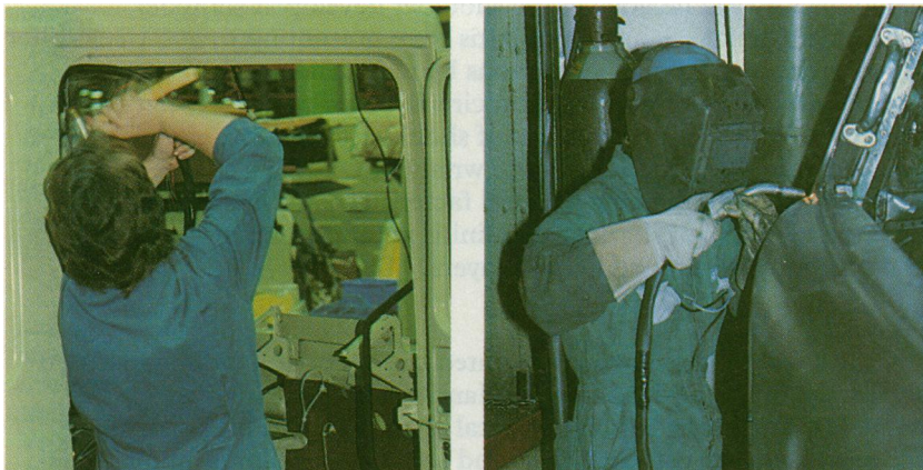
Truck assembly and welding—two jobs that often require working with the hands above shoulder height and that are associated with shoulder tendinitis.
