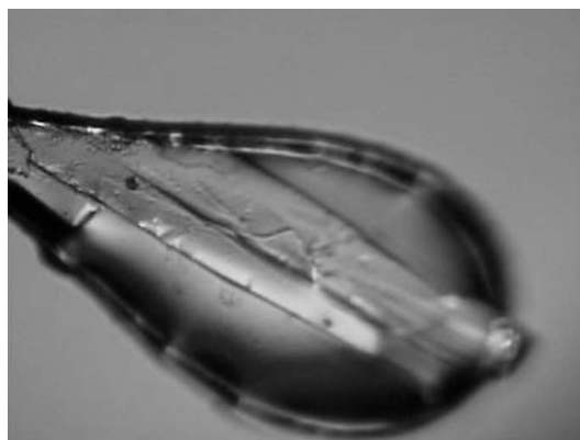
Figure 3 A native TnBgl3B crystal in the X-ray beam at beamline ID29 of the ESRF. The length of the crystal is approximately 400 μm.
