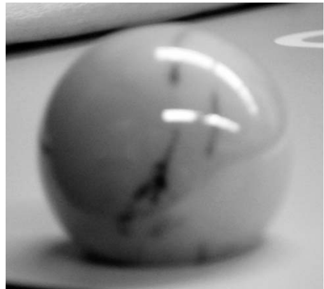
Fig. 1 The photograph shows a 36-mm ceramic femoral head, retrieved during bearing exchange revision for squeaking. Gray stripes are visible on the surface; scanning electron microscopy revealed these stripes were titanium deposits.
