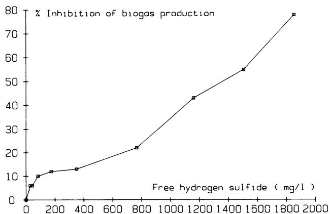
FIG. 5. Effect of free H 2 S on methane production from anaerobic digestion of medium A.
