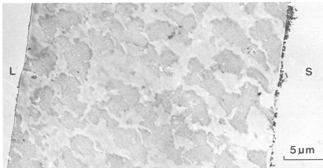
FIG. 2. Wall cross-section of an isotropic microporous polypropylene hollow-fiber membrane. L, Fiber lumen; S, shell space.
