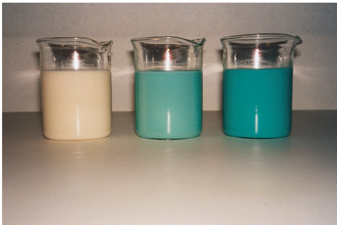
Figure 1. Dye-stained formula. At left is a beaker containing the formula, but no dye. In the center is a beaker containing the formula and FD&C Blue No. 1 dye at a concentration of 0.8 mL/L. At right is a beaker containing the formula and FD&C Blue No. 1 dye at a concentration of 1.5 mL/L.
