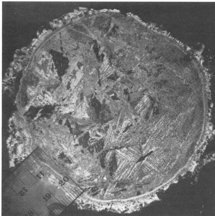
FIG. 2. Photograph of a horizontal section of an ice core. The section was located 5 cm from the bottom of core collected from annual sea ice in McMurdo Sound near the Ross Ice Shelf (IS, Fig. 1) on 10 November 1980. Light areas are cross sections of ice crystals. Between ice crystals are rows of liquid-filled brine channels (arrow) in which SIMCO were observed by phase-contrast microscopy. Centimeter marker is shown in lower left corner.
