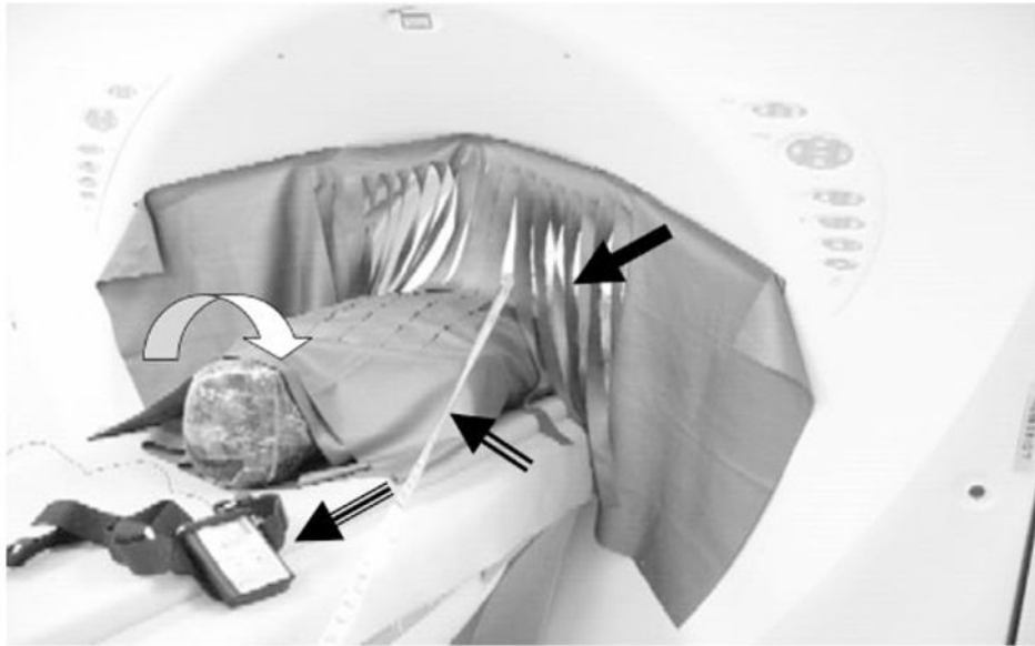
Figure 1. The fenestrated curtain drape (closed arrow) hangs from the CT gantry. The phantom is wrapped in a 360° double layer of shielding. The tape measure (two-line arrow) is used to determine the distances from the scan plane. The curved white arrow indicates the phantom head; the three-line arrowhead indicates the dosimeter.
