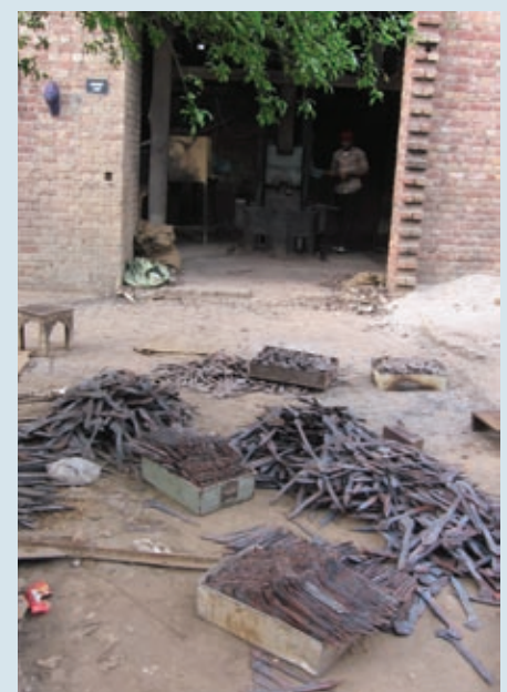
Surgical instruments in the courtyard of a forge in Pakistan before they are sent for polishing
