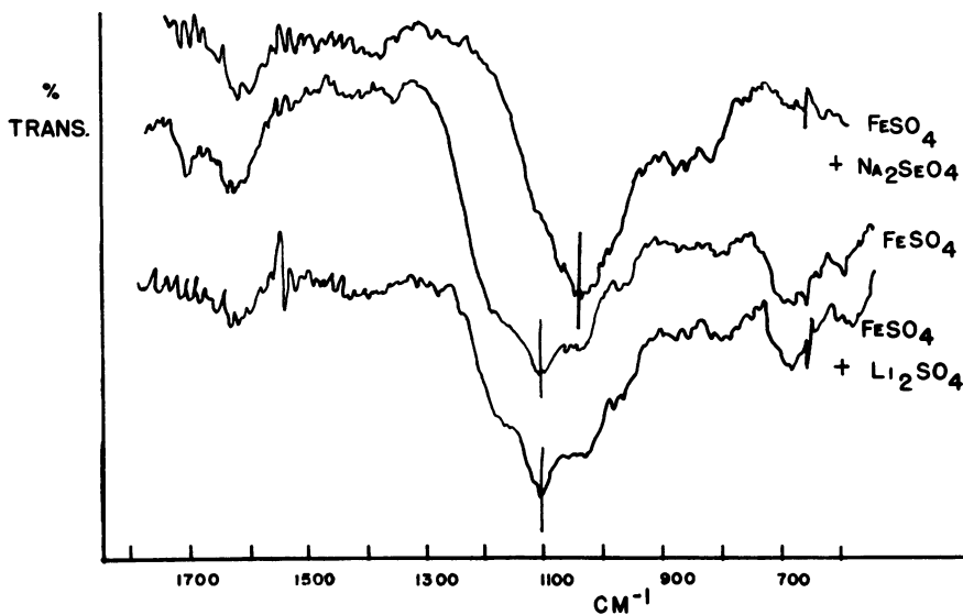
FIG. 6. Comparison of the IR spectrum of a partially selenated amorphous precipitate, formed by bacterial oxidation, with nonselenated amorphous bacterial ferric hydroxysulfate precipitates. The shift of major absorbance from \approx 1,115 \text{ cm}^{-1} in the amorphous sulfate to \approx 1,045 \text{ cm}^{-1} in the partially selenated analog is interpreted as the partial loss of sulfate activity at \approx 1,115 \text{ cm}^{-1} unmasking \delta(\text{OH}^-) absorption at \approx 1,045 \text{ cm}^{-1} .
