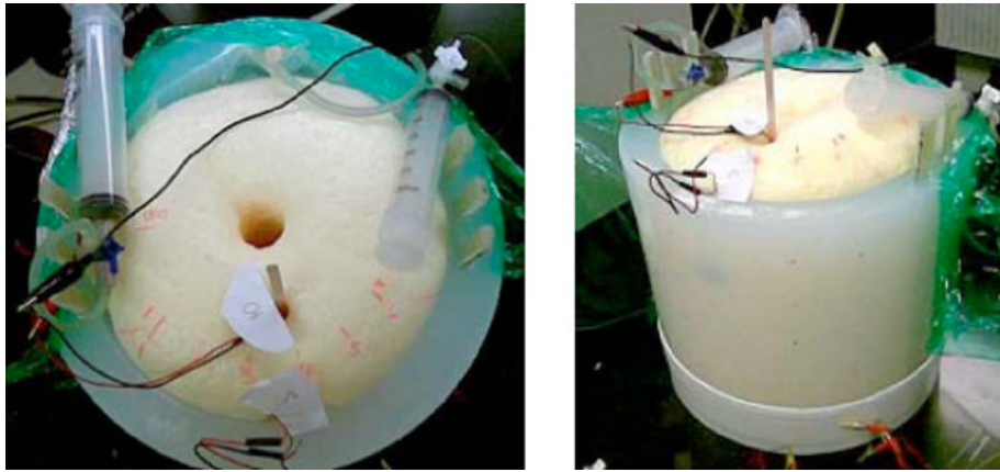
Fig. 6. Photograph of lung and chest wall mechanical phantom. Top and side views. Images show syringes that are used for inputting air into the bladders.
