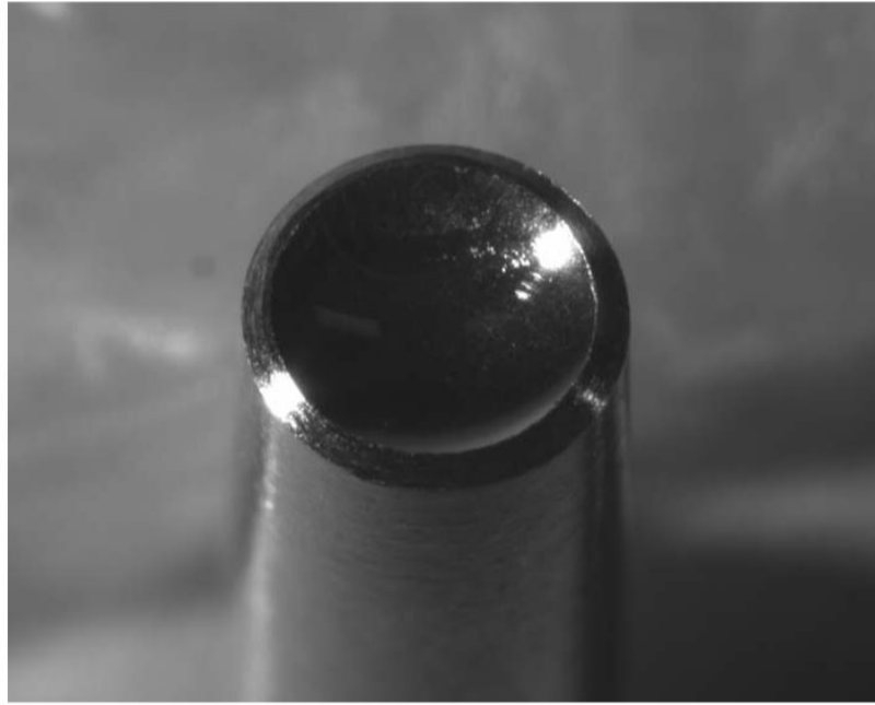
FIG. 1. A photograph of the spherically polished end of an aluminum rod that was used as the backing substrate for the transducers.
