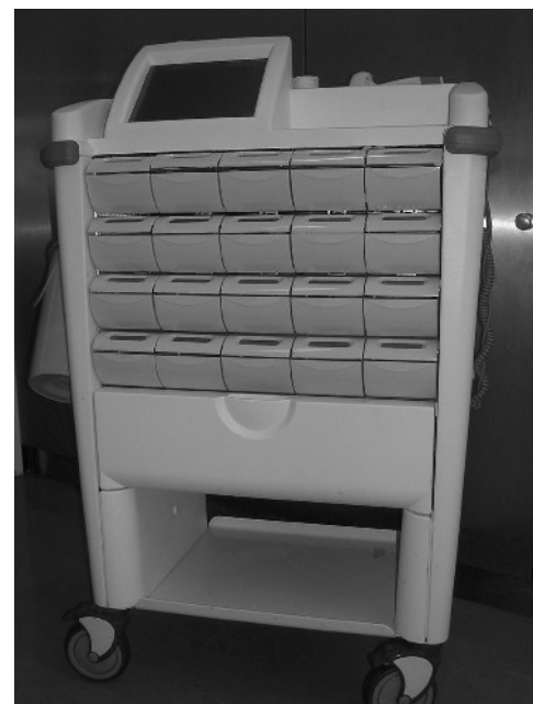
Figure A3 One of the two electronic drug trolleys. One drawer is allocated to each patient for whom medication is due and their name shown on the liquid crystal display. The barcode scanner is on the top of the trolley.
