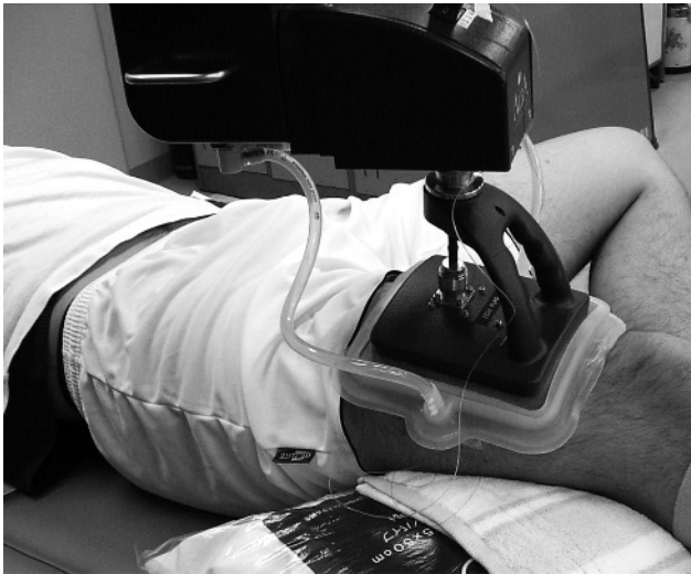
Figure 1 The applicator for the hyperthermia system positioned on a human thigh. Informed consent was obtained for publication of this figure.
