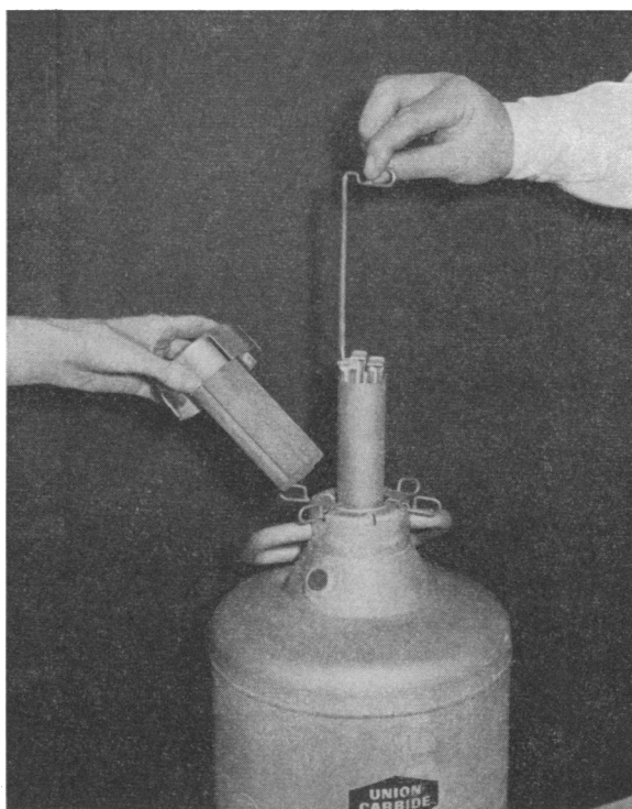
FIG. 4 INSERTION OF CANISTER INTO REFRIGERATOR-TRANSPORTER
