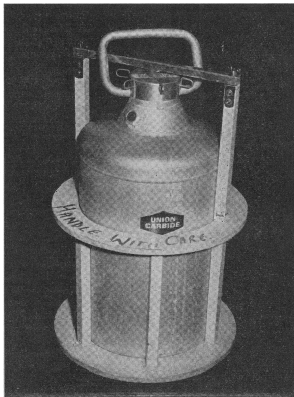
FIG. 1 EXTERNAL ASPECT OF LIQUID NITROGEN REFRIGERATOR-TRANSPORTER
