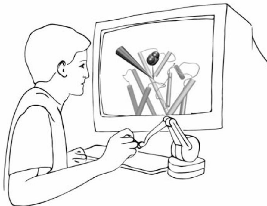
Figure 7. In IMD, the user applies forces to atoms in the simulation via a force-feedback haptic device.
