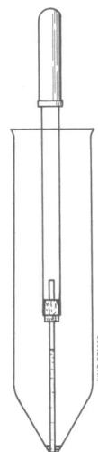
Fig. 1. Pipetting device to draw previously centrifuged cerebrospinal fluid (CSF) sediment into a capillary tube for further centrifugation.
