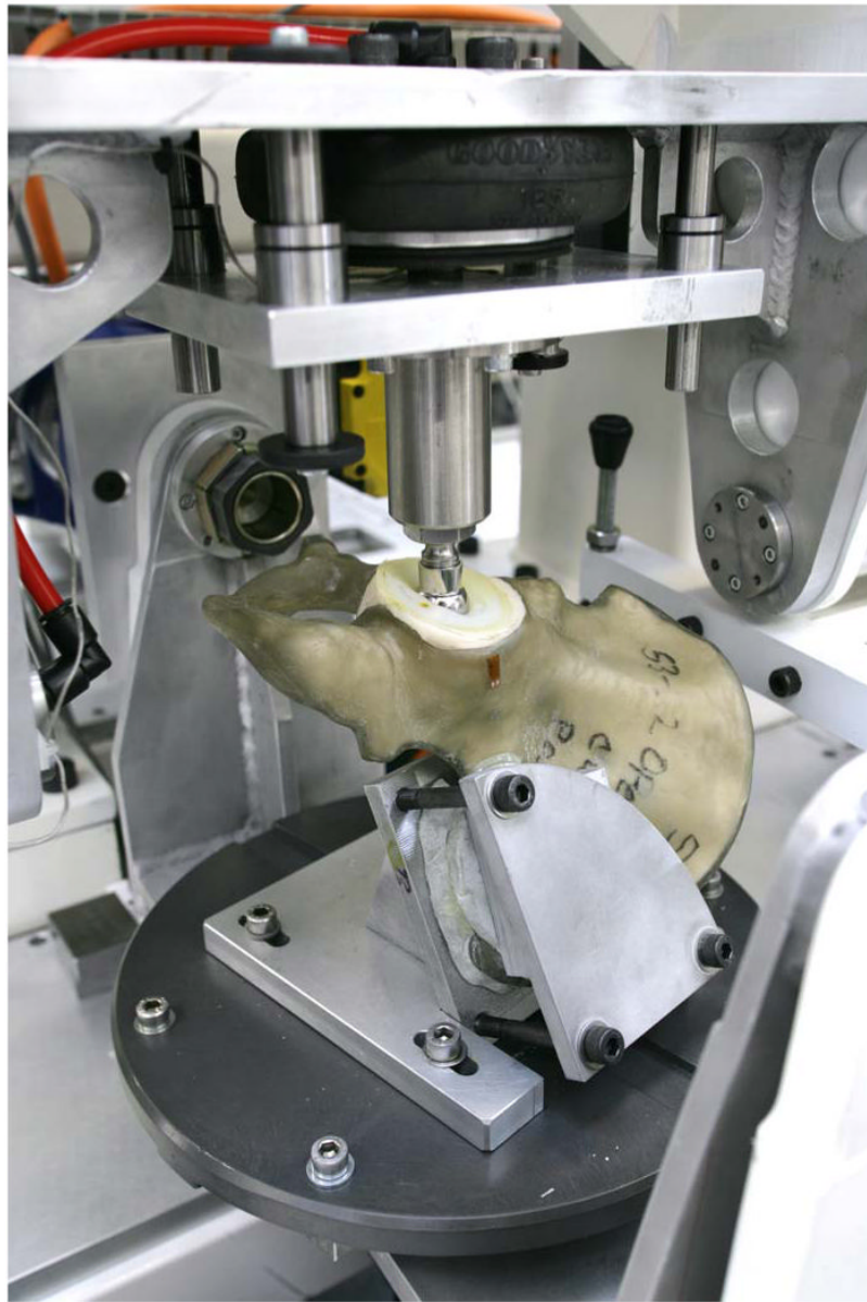
Fig. 3. The Portsmouth four station hip simulator with a specimen loaded in one of the test cells
