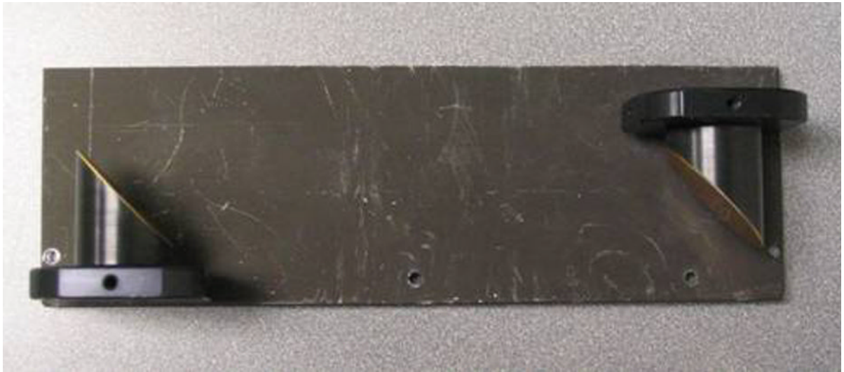
Figure 8. An astronomical Keplerian prototype telescope constructed from two 90^\circ off-axis parabolic mirrors.
