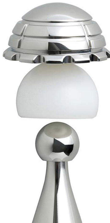
Fig. 1 The cemented Medial Cup ® DMC consists of a steel inox polished spherocylindrical cemented metal cup and a PE cup insert. Flexion occurs mainly in the small inner articulation. Abduction/adduction and rotation start in the small articulation (up to 25°) and continue up to 54° in the large peripheral articulation between the PE cup and the metallic socket. The PE cup ( \geq 8 -mm thickness) is not constrained in the metallic socket (no retentive rim), but the PE inner articulation is retentive. The femoral head, usually metallic (22 mm), is clipped inside the PE cup intraoperatively.
