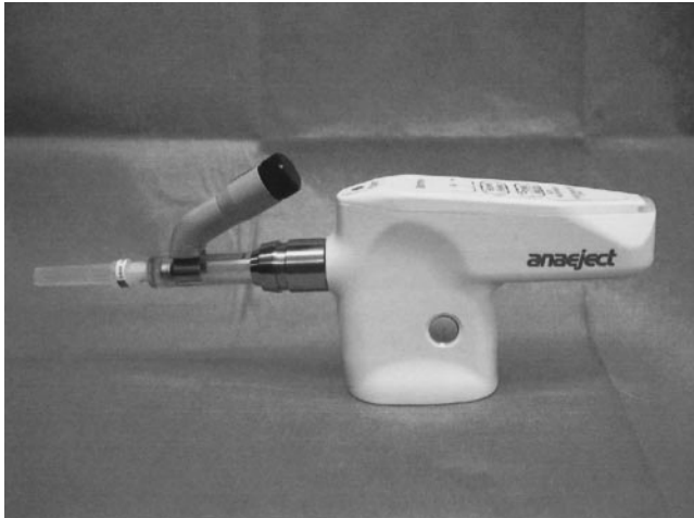
Figure 1. Setup for connecting Vibraject to Anaeject.
