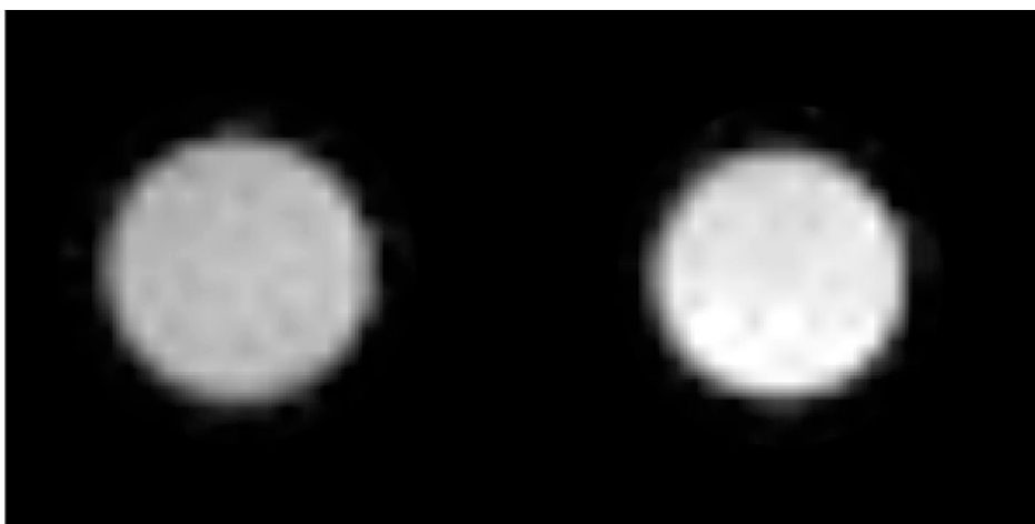
Fig. 8. Internalized quantum dots produce MRI contrast. T1-weighted images from tubes containing cell lysates show that lysates of cells that have been incubated with quantum dots (right) show significant contrast enhancement compared to cells that have not been exposed to quantum dots. These samples were from cells in the same experiment shown for the optical uptake studies of Fig. 6 and Fig 7. Images are 0.5 cm in diameter.
