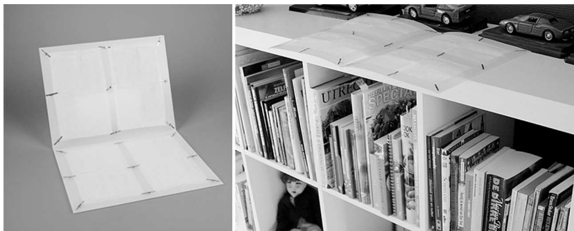
FIG. 1. The EDC. The sampler consists of four electrostatic cloths mounted in a 40- by 30-cm plastic folder that is left for 14 days in the horizontal position with the cloths exposed to the air. The folder is kept closed before and after sampling and during transport and storage.
