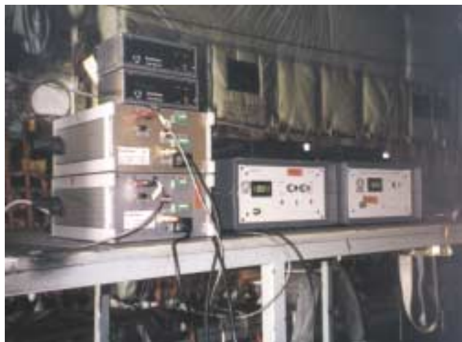
Figure 6. Photograph of the real-time PAH monitors in the cargo bay of a C-130H aircraft during an ERO-loading exercise on 6 May 1999.
