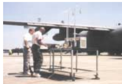
Figure 1. Photograph of the sampling equipment positioned downwind from a C-130H aircraft during a four-engine run-up test on 4 May 1999.
