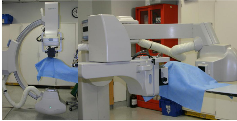
Figure 10. HSMAF system in horizontal and vertical angles during ROI-CBCT acquisition of a stent in a rabbit.
