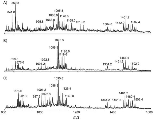
FIG. 4. MS analysis of intact LOS after microwave-assisted protease K digestion for 1 min (A), 3 min (B), and 5 min (C). The analysis conditions were the same as those for Fig. 2.
