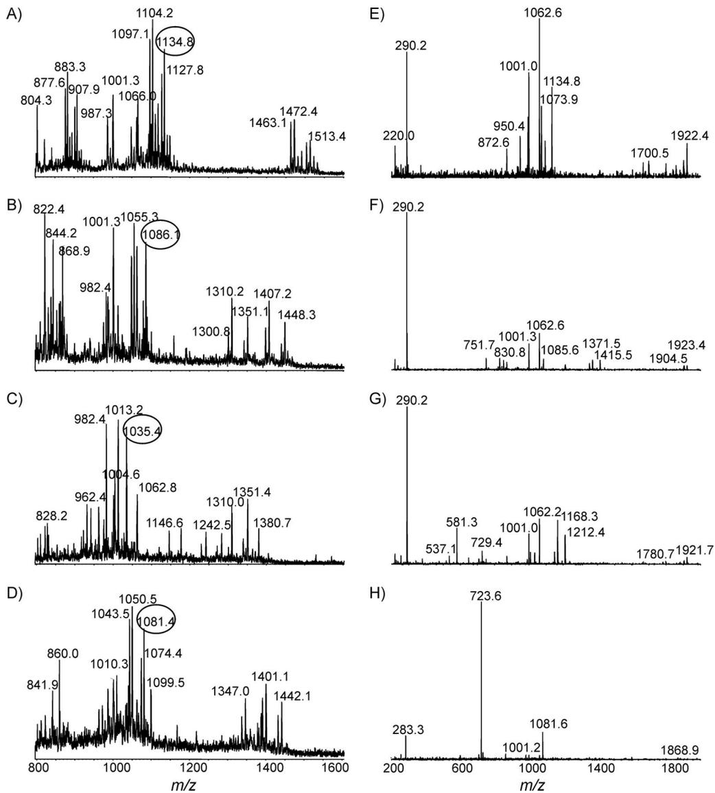
FIG. 8. EA-OTLC-MS and EA-OTLC-MS/MS of intact LOS. All experimental conditions were the same as those for Fig. 3. (A) Strain GB13; (B) strain GB11; (C) strain MF8; (D) strain GB4; (E) product ion spectrum with an  $m/z$  of 1,134.8 ( $[M-4H]^{4-}$ ); (F) product ion spectrum with an  $m/z$  of 1,086.1 ( $[M-4H]^{4-}$ ); (G) product ion spectrum with an  $m/z$  of 1,035.4 ( $[M-4H]^{4-}$ ); (H) product ion spectrum with an  $m/z$  of 1,081.4 ( $[M-4H]^{4-}$ ).
