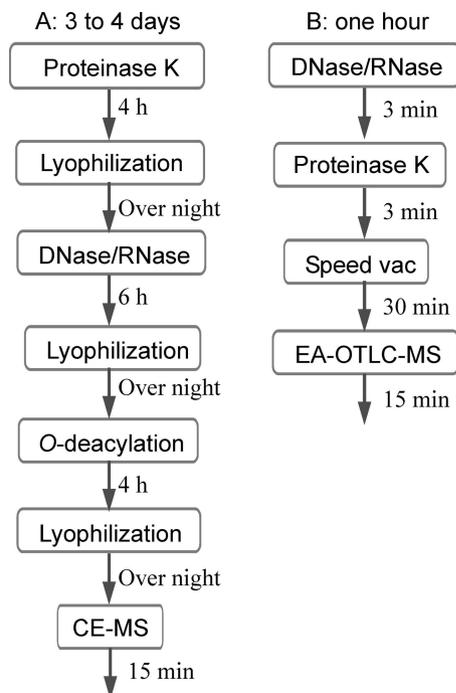
FIG. 1. Illustration of sample preparation procedures. CE-MS, capillary electrophoresis-MS.
