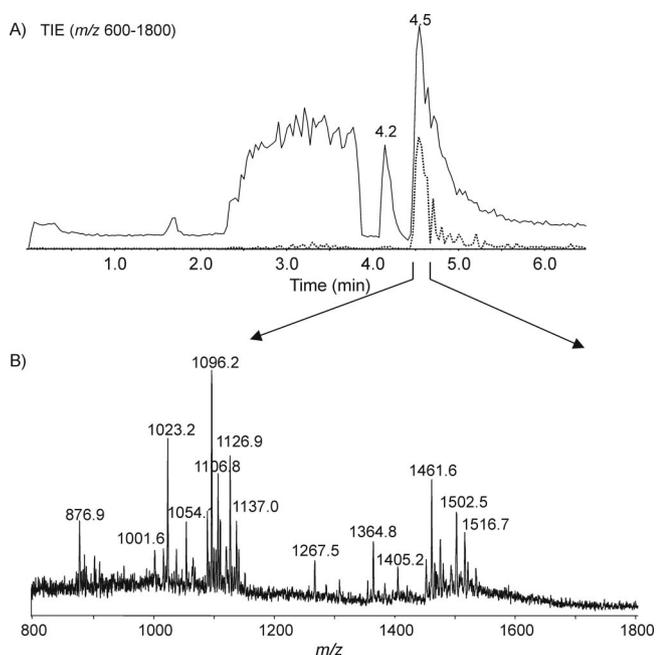
FIG. 2. EA-OTLC-MS analysis of intact LOS from *C. jejuni* MF6 prepared using a traditional method. A separation voltage of 20 kV, together with a pressure of 50 kPa, was employed. Samples (1.0  $\mu$ l) were injected. (A) Total ion chromatogram ( $m/z$  values of 600 to 1,800) and extracted ion chromatogram ( $m/z$  of 1,096.2); (B) extracted mass spectrum at 4.5 min.
