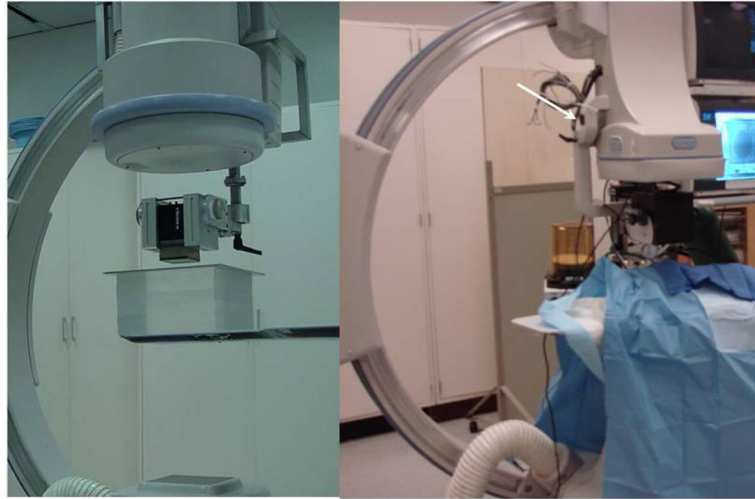
Figure 2. Micro-Angiographic detector mounted on a standard C-Arm with XII (left) and HSMAF mounted with FP (right). The images acquired with the HSMAF detector are automatically displayed on a monitor adjacent to the flat panel monitors. The automatic collimation button (white arrow in the right image) is attached onto the HSMAF holder
