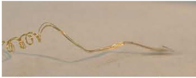
Figure 8. View of the glass cone tip containing four wires.
