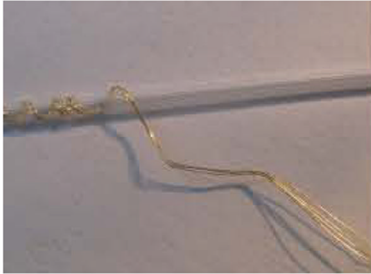
Figure 4. Forth-five degree bends in coiled wires that limit depth of cone tip insertion.
