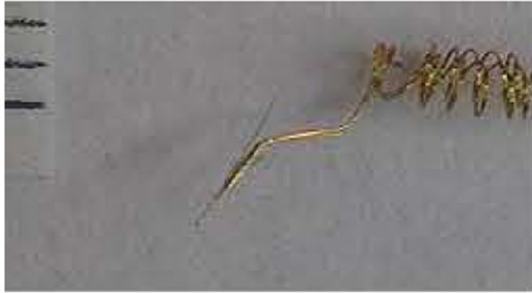
Figure 7. Glass cone tip is maneuvered onto three gold wires using a piece of hair as a “handle”.
