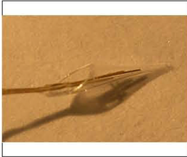
Figure 9. The cone tip has a shelf for gluing wires securely into position.
