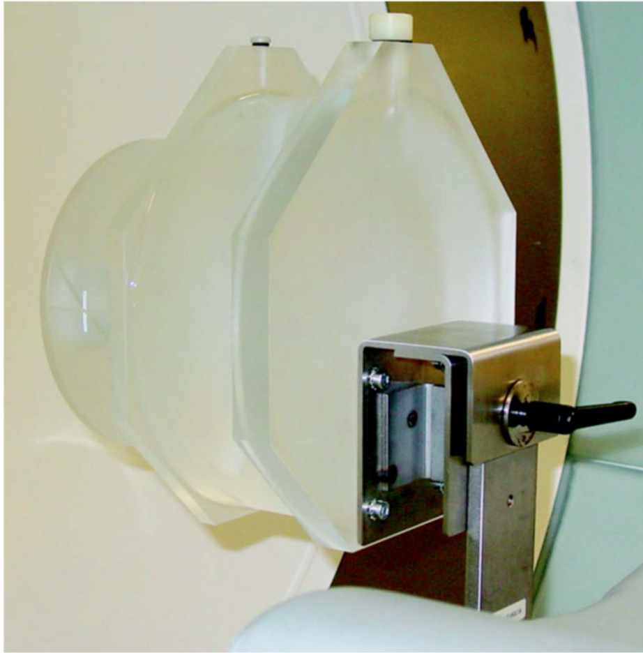
FIG. 1. A phantom used for daily water calibrations of the scanner. The water-filled, 20 cm diameter section of this phantom was used. The cantilevered design ensures no table attenuation is present in the scan plane.
