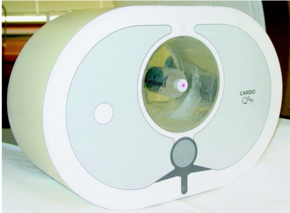
FIG. 2. An anthropomorphic cardiac phantom (QRM, Möhrendorf, Germany) with its central portion replaced with a water-filled tank. The syringe centered in the middle of the tank was filled with water and iodine solutions.
