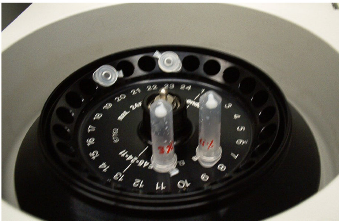
Figure 1. 2-ml volumes of the emulsions were centrifuged for 30 minutes at 16K \times g to remove large aggregates formed during the polymerization process. The compacted pellet obtained after removal of the supernatant is shown.
