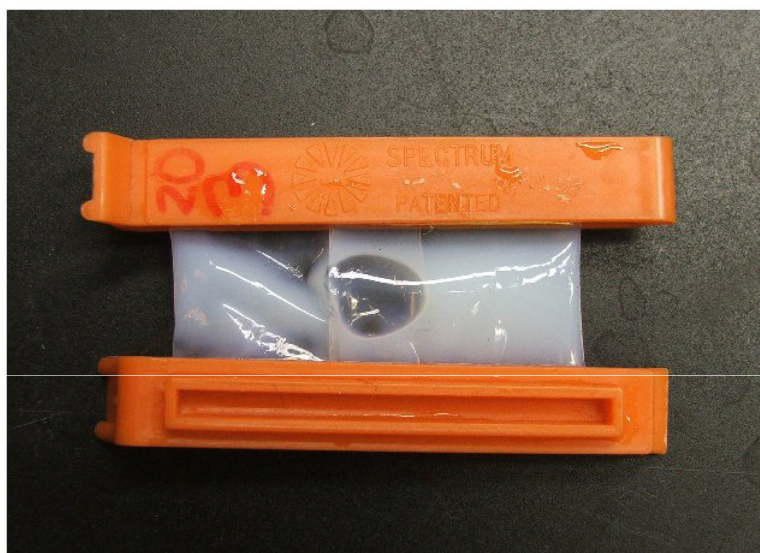
Figure 2. Dialysis of the emulsion was conducted with different dialysis membranes (MWCO's of 6–8K, 12–14K, 50K and 100K) and dialysis times (4–24 hours) in bulk water.
