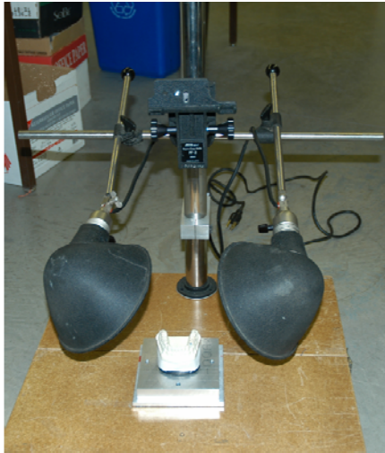
Fig. (3). Photographic set up—camera placed at 90° directly over cast.
