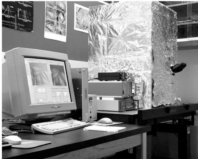
Fig. 6. An overview of a thermal-stable microscope that we use in our research. The microscope proper is mounted on a vibration-isolation table and is equipped with filter wheels, multiple shutters, and a Rose-chamber stage heater. All of these devices are covered by a cardboard box (covered with aluminum foil), to shield the entire assembly from airflow and light. Electronic controllers for all of these devices are placed outside of the microscope to prevent their overheating. The whole system is driven by a workstation (on the left) that runs image-acquisition software (in this case Isee, Isee Imaging, Raleigh, NC, USA).
