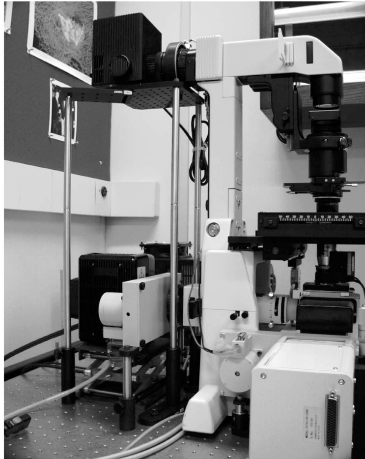
Fig. 2. Vibrations generated by shutters and filter wheels can be eliminated by mounting such devices external to the microscope chassis. In this example, the shutter/epi-light source assembly and filter wheel (bottom), as well as shutter/trans-illumination source assembly (top), are all mounted onto a vibration-isolation table using stainless steel rods. The whole assembly is disconnected from the microscope body, which in turn rests on the same vibration-isolation table.
