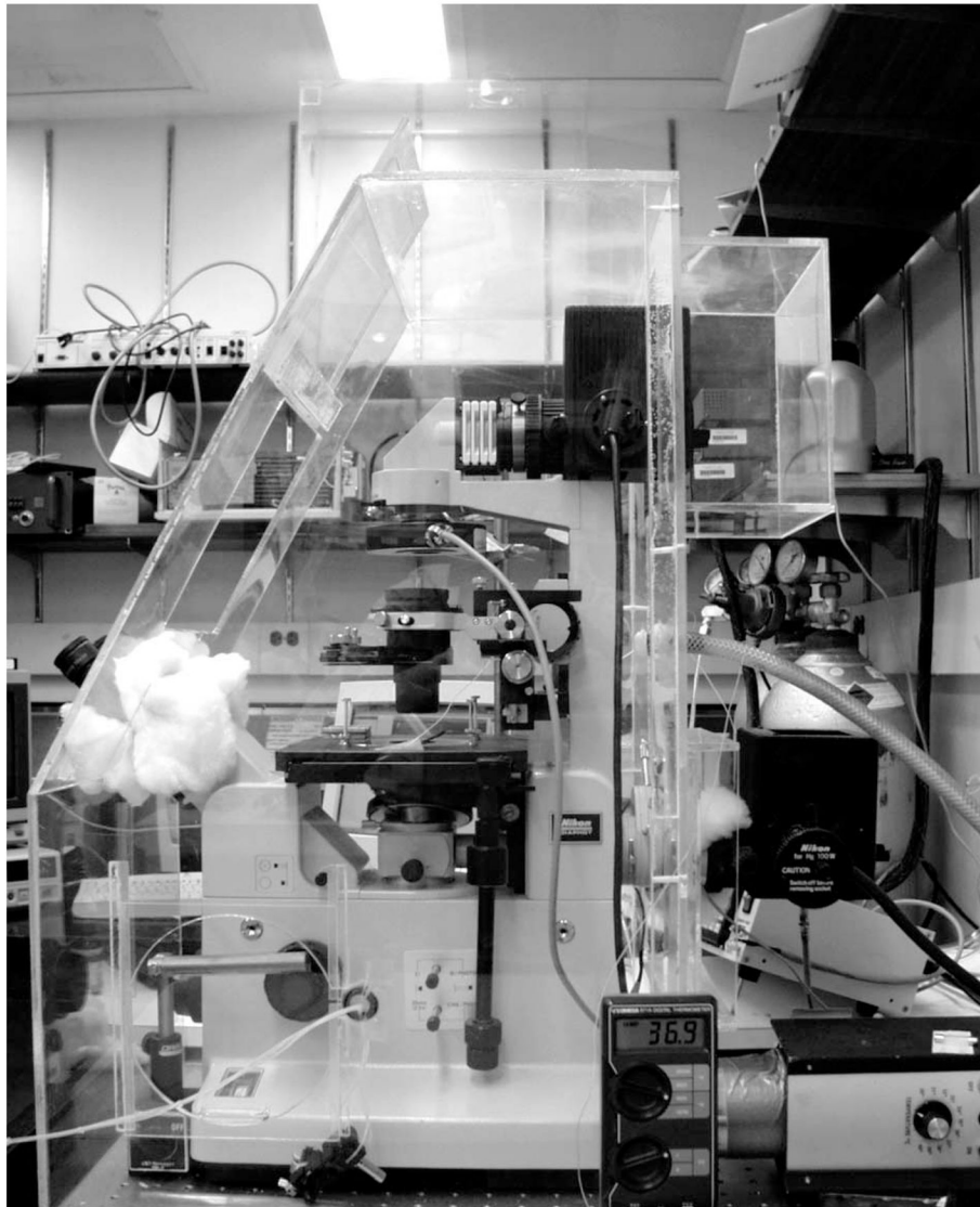
Fig. 4. Enclosing the microscope and some of its peripherals in a plexiglass box allows for precise control of the specimen temperature during live-cell imaging. The temperature inside of this box is maintained by a heat blower (bottom right hand corner of image), positioned well away from the specimen stage, which cycles on and off in response to a thermistor positioned near the specimen. Note that the oculars protrude from the box (but are sealed by cotton), and that focusing can be done externally. See text for details.
