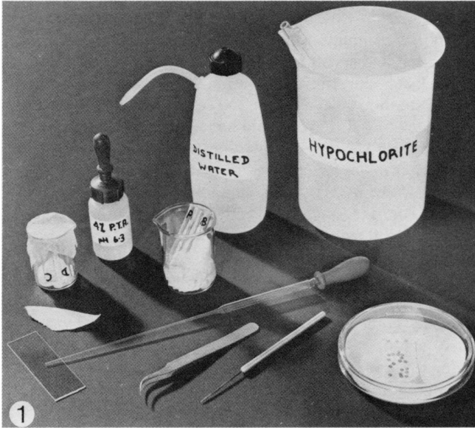
PLATE 1. The equipment needed to carry out negative staining. Note that specimens waiting to be examined are contained in a beaker sealed with parafilm and are still inverted. Those already dealt with are in the open beaker.
