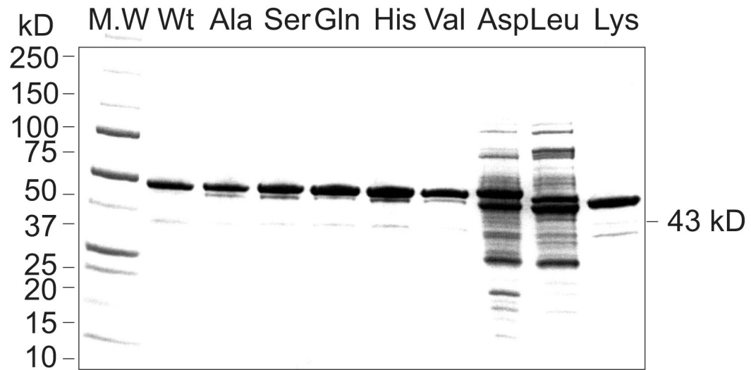
Fig. 2. SDS -PAGE with Coomassie staining of wild type cAOS and its mutant proteins after Ni- NTA affinity chromatography. Each lane was loaded with 1–2 \mu\text{g} of protein, except for the Asp and Leu mutants, which were loaded with \sim 4 \mu\text{g} protein due to their lower levels of cAOS expression in E. coli .
