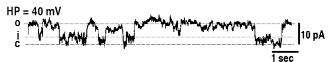
FIGURE 6 Unitary channel recording obtained in liposome-attached configuration of the patch-clamp technique. Shown is a representative current trace recorded at 40 mV (holding potential, HP ) from a patch containing one active channel under symmetrical conditions (150 mM KCl inside and outside the liposome). The open, intermediate, and closed states of the channel are indicated with dotted lines and the letters O, I, and C, respectively.
