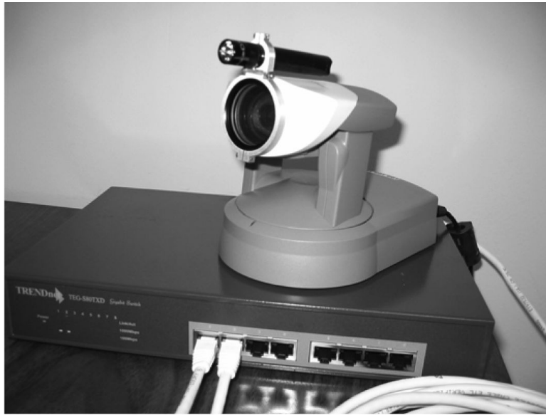
Fig. 3. One of the Axis Network Cameras shown sitting on top of the hi-speed switch to which all cameras are attached when in use. On top of the camera is an LED light source. The light source is mounted to the camera, as shown, and moves with the camera during pan and tilt operations.
