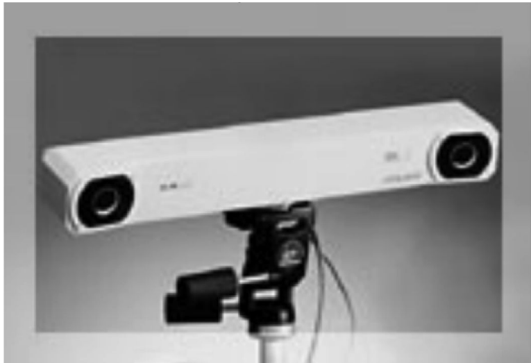
Figure 7. The Polaris IR tracking device. The black rings contains many IR-emitting LEDs. One IR camera is located at the center of each LED ring.
