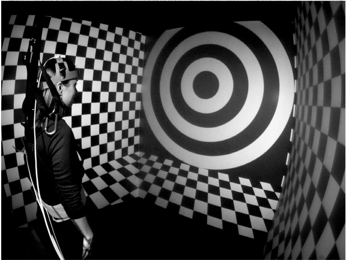
Figure 1. Subject standing in full field of view Balance NAVE Automatic Virtual Environment, consisting of three adjacent screens that surround the subject and encompass 180° of the horizontal and 70° of the vertical field of view. Entire visual image moves in anterior-posterior direction at 0.4 Hz during optic flow stimulation.
