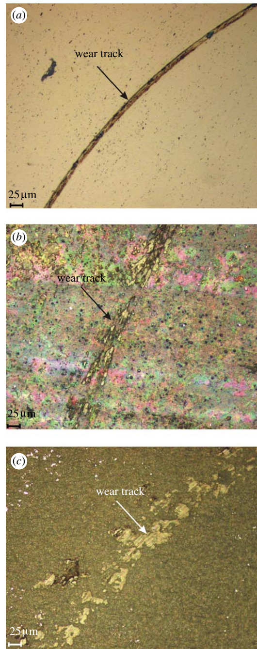
Figure 8. Images of the surfaces after nanotribo test. (a) Polished surface, (b) alkali-treated and (c) spark oxidized nitinol samples.
