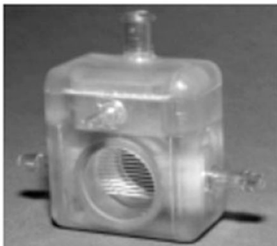
FIGURE 2. Bioreactor incorporates two external fluidic systems, O-ring sealed caps, and a sample reservoir. 28 Used with permission from ProBioGen AG.
